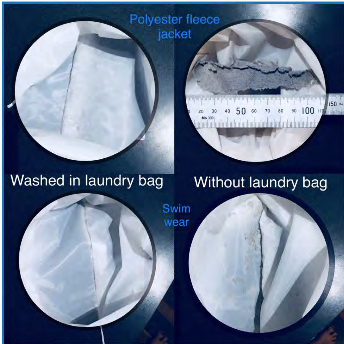
Figure 18. Image of microfibrils released in laundry waste water for aged polyester fleece jackets and aged swim-wear when washed with and without a laundry bag, in a front loader machine. For fleece jackets microfibre yield was reduced 91%, for swim-wear microfibre yield was reduced 87%.
