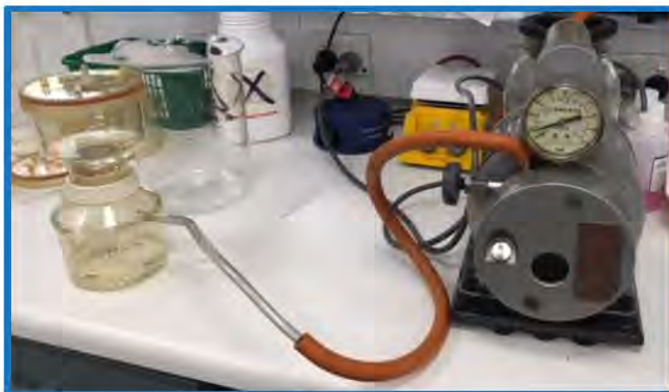
Figure 8. Filtration equipment for laundry trial: 25 µm filter bag, filter housing, using 1.2 µm paper filters and pump.
