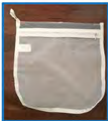
Figure 7. Laundry bag made from 50 µm monofilament nylon.
