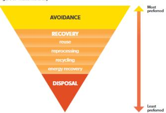
Resource recovery options recover value from materials, thereby offsetting the environmental impacts of extracting and processing raw materials. Energy recovery is the least preferred recovery option.
