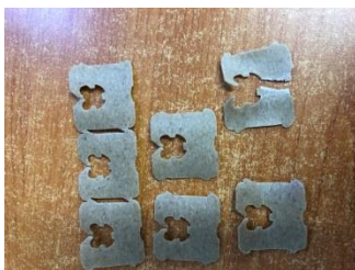
Figure 7 Cliplocks made from compostable material. Shown warped and broken when exposed to moisture and pressure.
