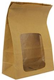
Figure 4 Example of one of the compostable - cellulose bags (with paper) that was trialed but failed as it could not withstand moisture.
