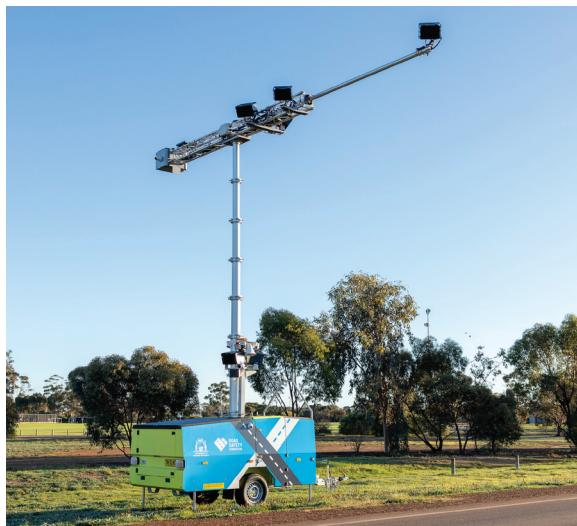
These new safety cameras are mounted on large, bright yellow trailers with Road Safety Commission branding. They can be moved to various locations and are able to operate continuously (24 hours a day) for several days if required. The safety camera trailers can detect:
