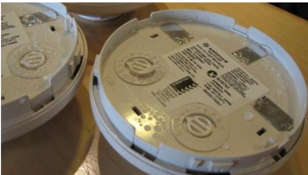
Figure 13 Condensation within smoke alarms cause false alarms
