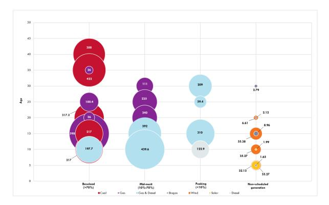
Figure 5: Facilities operating in the SWIS by age, fuel capability, and classification<sup>21</sup>
