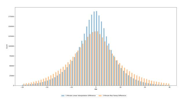
Figure 11: Differences between actual load and ramping profiles – CY 2018
