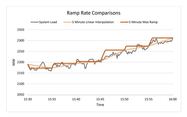
Figure 10: Ramp Rate Comparisons, beginning of evening ramp on 18/10/2018
