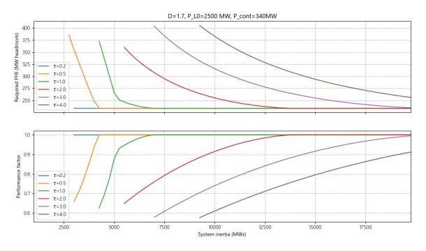
The top panel shows the system secure zone if all reserve were sourced from facilities with the same speed factor, for a range of speed factors. Traditionally, the WEM has been operated with an assumption of  $\tau = 2$ . With different speeds of connected facilities, the secure zone changes:
