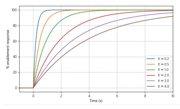
A facility which can provide full response within a fraction of a second might have a  $\tau = 0.2$ , while a facility that takes several seconds to fully respond might have a  $\tau = 4$  (that is, the lower the  $\tau$  factor, the higher the speed factor).
