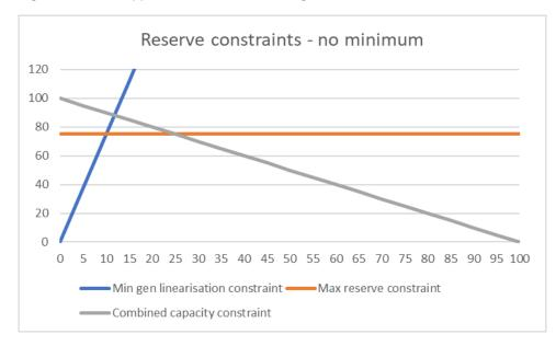
Figure 8: Linear approximation of minimum generation constraint
