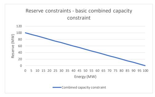
Figure 6: Joint capacity and maximum reserve constraints
