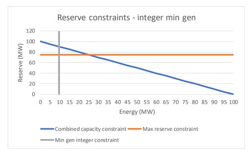
Integer problems are much harder to optimise than those involving linear variables only, as the solution space is not continuous – the clearing engine must either choose to dispatch the facility for 0 energy and 0 reserve, or for some point under the curve. As a result, solve times for integer problems are longer than linear problems, and can vary considerably depending on input parameters. A second (linear) run is required to determine prices.
