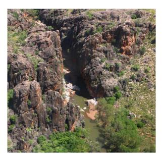
This hydraulic model required a high resolution digital elevation model (HRDEM) to define the geometry of the gorge. In developing the model, we used a drone and image recognition technology to capture a point cloud (a set of data points in space) of more than 83 million ground points. We used GIS software to post-process the point cloud to produce an HRDEM suitable for our purposes.
