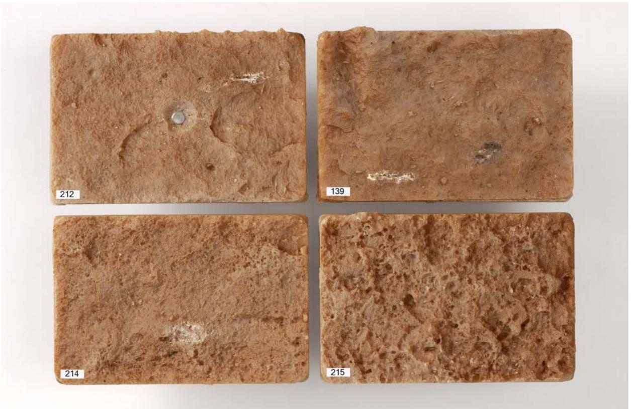
**Figure 33: Tiles after exposure (12 months) Site 5; Burrup Rd.**
