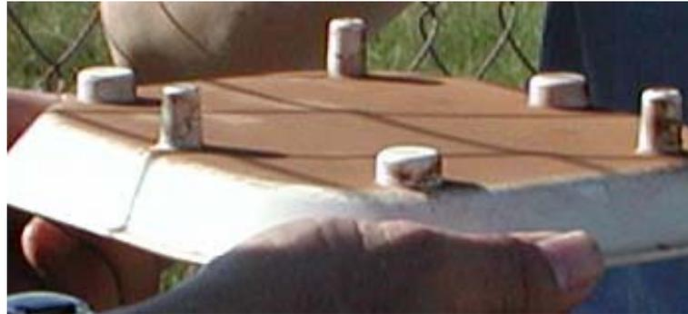
Figure 26: Dust deposited on datalogger housing.
