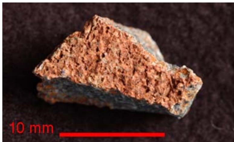
Figure 19: Optical microscopy of rock subsample prepared for fumigation.
