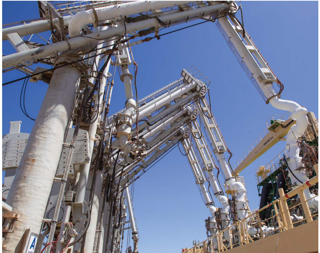
Loading arms transfer LNG to vessel ahead of first cargo sail-away at Chevron's Wheatstone Project. Photo: Chevron
