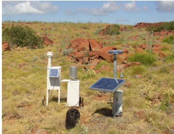
Figure 4 Microvol sampler and rainwater sampler at Dolphin Island (Source: CSIRO 2010a)
