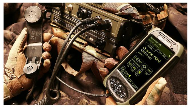
Western Australian company Barrett Communications designs and manufactures a range of high frequency and very high frequency products, featuring the latest in communication technologies. Pictured is a Barrett PRC-4090 Tactical HF software defined radio. **Photo credit:** Barrett Communications
