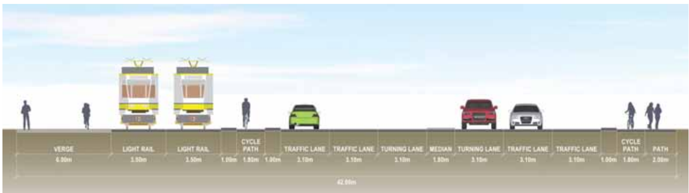
Figure 35: Stephenson Avenue Conceptual Cross Section – Stephenson Bridge
