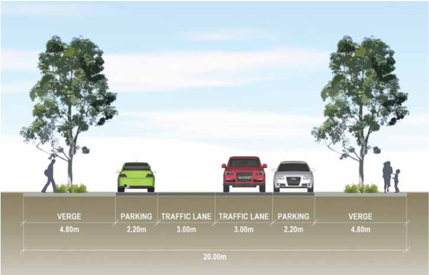
Figure 41: Howe Street Conceptual Cross Section (between King Edward Road and Stephenson Avenue)
