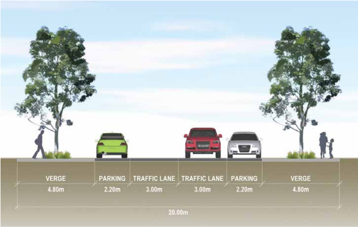
Figure 52: Guthrie Street Conceptual Cross Section
