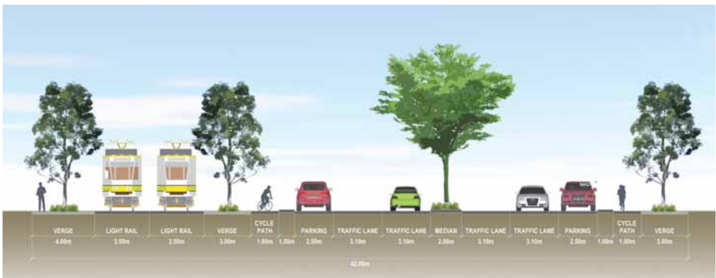
Figure 36: Stephenson Avenue Conceptual Cross Section – Freeway to Guthrie Street
