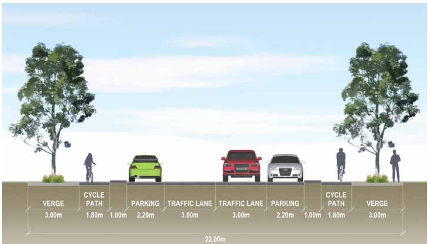
Figure 56: Liege Street Cross Section
