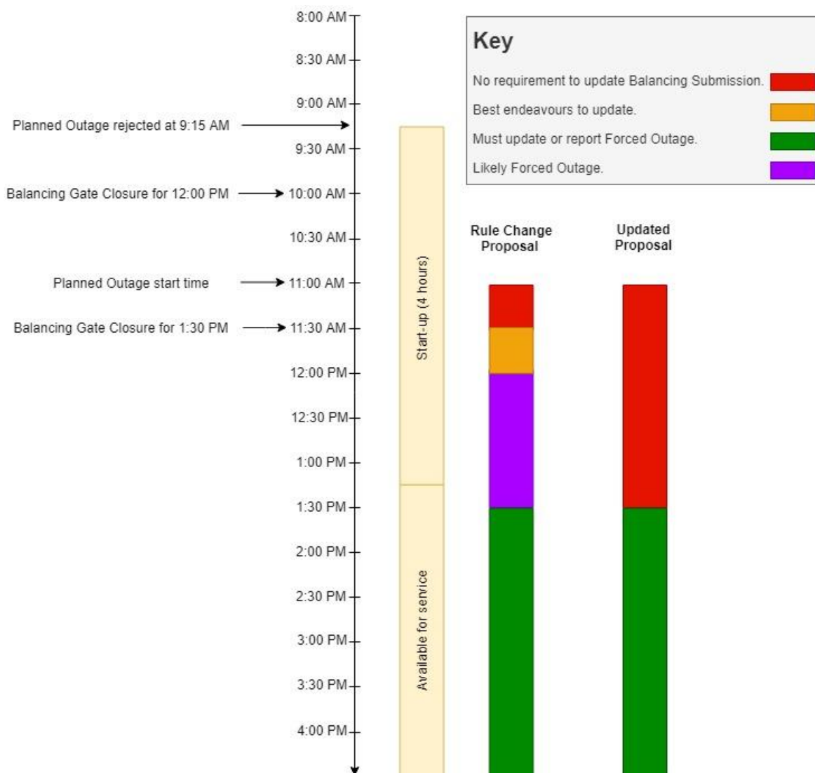
Figure 6.2: Late rejection of a Planned Outage – Balancing Facility with a 4-hour start-up time
