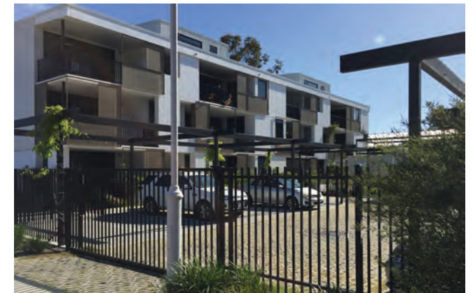
Photo G3.4b This secure communal parking area incorporates permeable paving and is co-located with other shared facilities, including community gardens and storage areas
