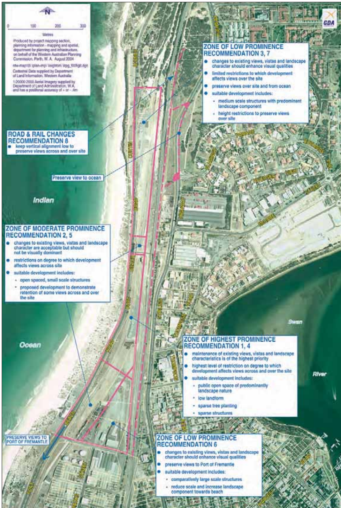
Figure 2.14: Example of a site level visual landscape strategy map, with recommendations grouped according to relative prominence of portions of the site.
