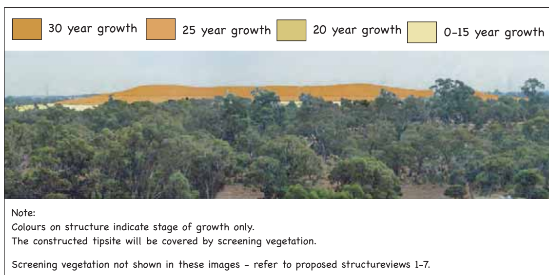
Figure 2.16: This figure from a Kwinana waste site proposal illustrates how a landform analysis could be graphically presented. Adapted from image supplied by Ecoscape Australia Pty Ltd.
