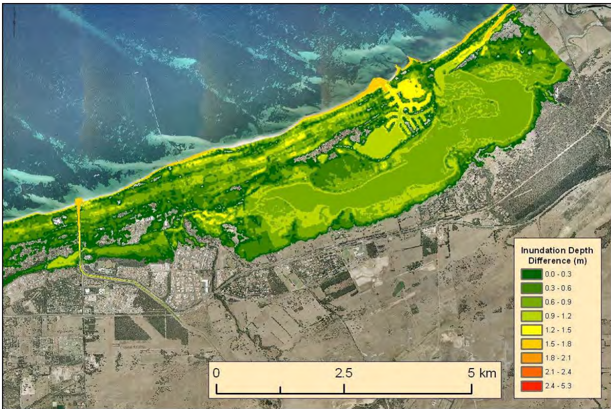
Figure 27. Difference in the inundation depth; B1 - B0.
