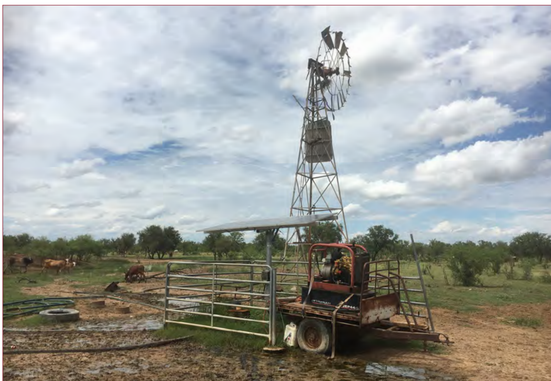
Figure 11: Example of a diesel pump at a bore as a temporary measure
