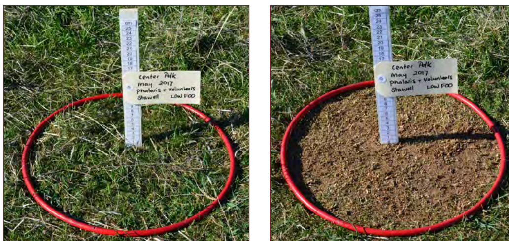
Figure 44: Calibration ring on green grass and trimmings of green feed for determining FOO
