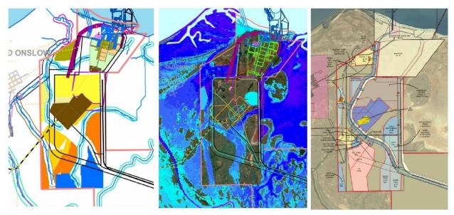
Figure 6 Series of report images showing how natural channels identified within the hydrological study (left and middle) (BG&E, 2011c) shaped part of the Stage 1B & 1C Development Plan (right) (TPG, 2012)
