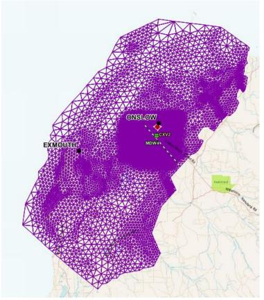
Figure 19 – Extents of model mesh representing the Birdrong Aquifer, used for the OWIUP study (Water Corporation, 2014a)
