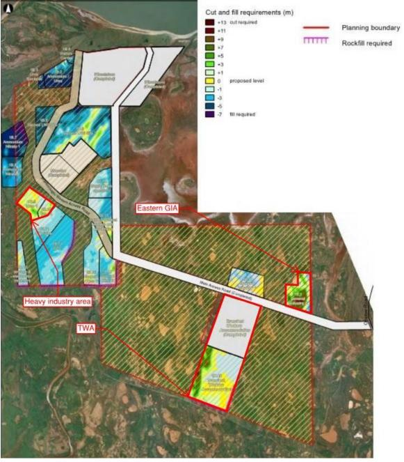
Figure 12 – Annotated extract of Fill Sourcing Study indicating cut-fill requirements from previous stages of the ANSIA, where green and brown indicates cut, blue indicates fill, and yellow is already balanced (Arup, 2014).
