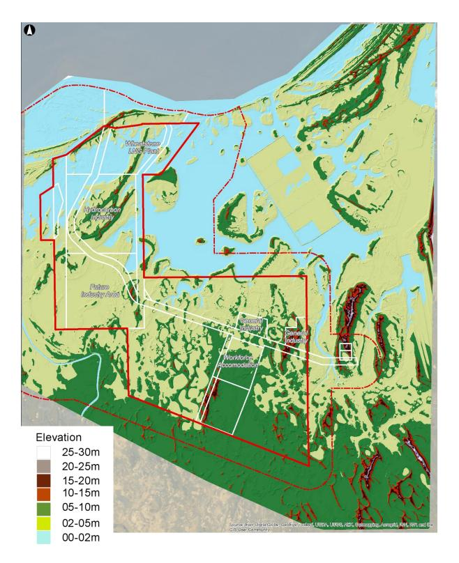
Figure 4 – GIS output showing Lidar elevations indicating low lying and natural high ground in relation to future areas of development at the ANSIA.
