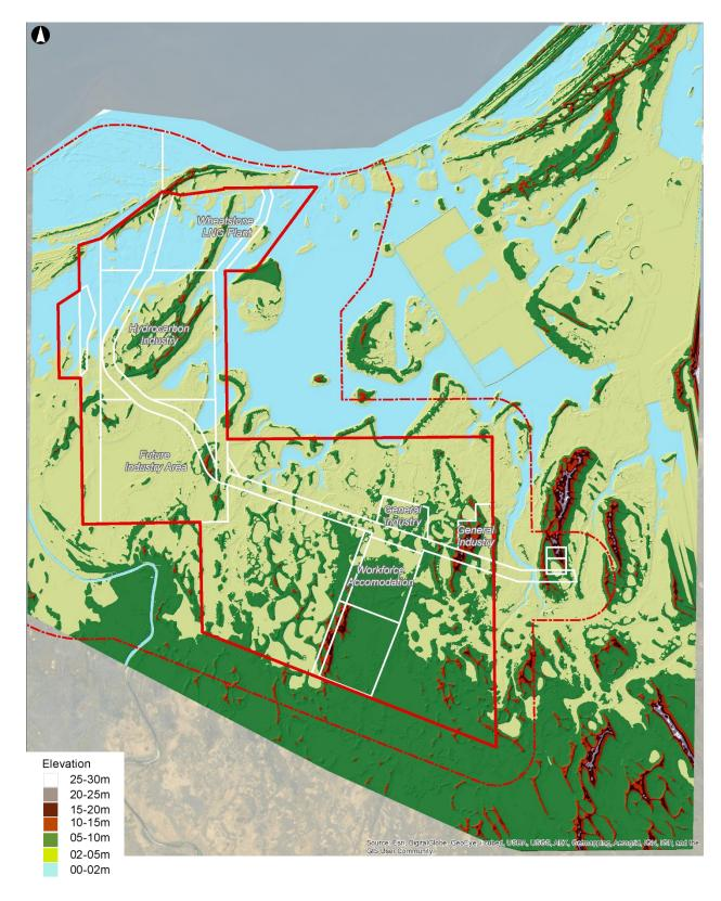
Figure 11 – GIS output of Lidar survey showing higher and low lying areas (m AHD) in relation to future stages of the ANSIA.
