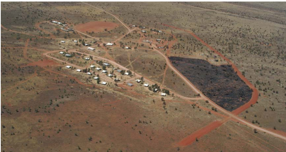
March 2003 looking south east – The red ribbon on the right is a drain/levy established to mitigate flooding
