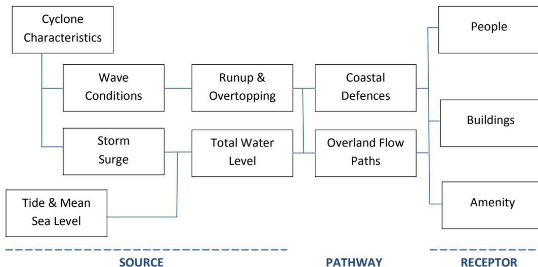
**Figure 6-2: Example of Source-Pathway-Receptor Factors for Inundation**
