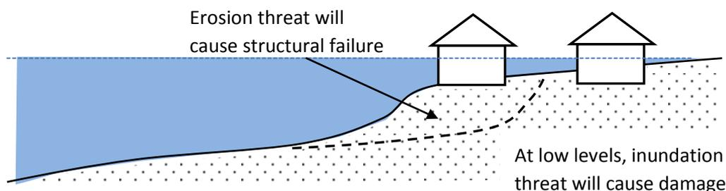
**Figure 6-4: Schematic Illustration of Erosion and Inundation Threats**
