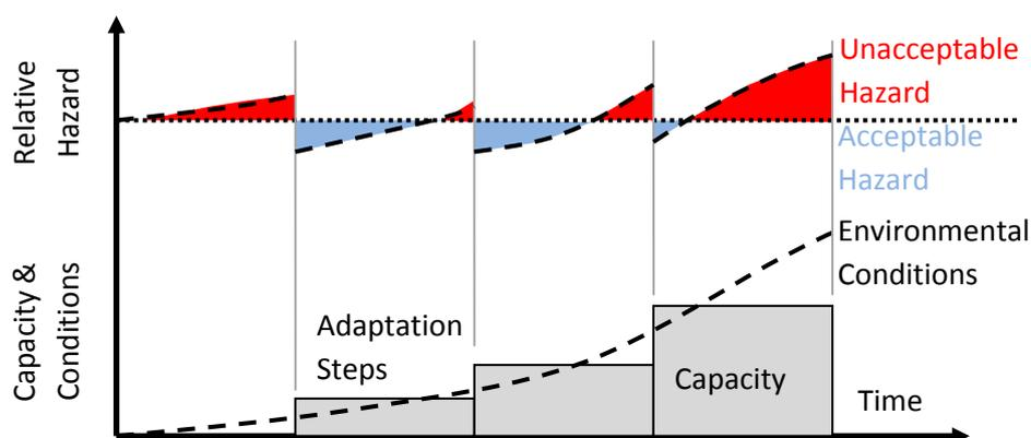
**Figure 6-5: Schematic of Hazard Sequence Associated with Adaptation Steps**
