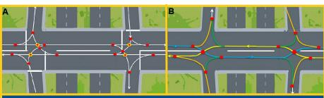
**Above** Figure A shows a standard WA interchange with 18 possible conflict points of which 4 are classified as causing serious injury. Figure B shows the layout of the DDI with 12 conflict points of which none are classified as serious thereby significantly reducing the potential for death and serious injury from vehicular impact.
