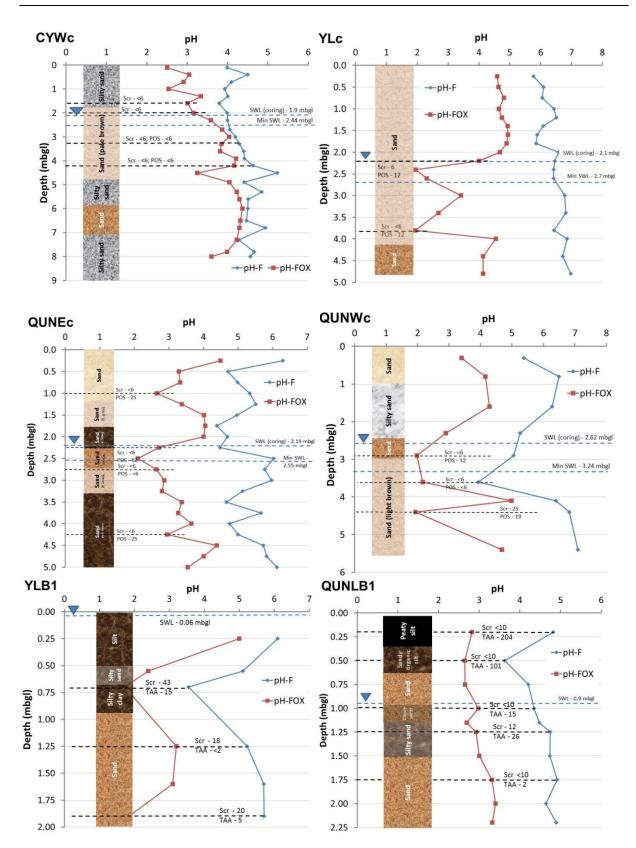
Figure 14 Field (F) and peroxide (FOX) oxidised pH, summary lithology and potential acidity analyses (moles H<sup>+</sup>/tonne) for superficial formations and selected lake beds at three north Yeal wetlands
