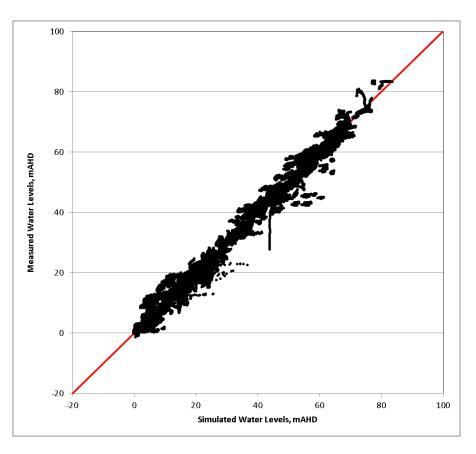
Figure 32: Calibration Error – Superficial Aquifer PRAMS 3.5B
