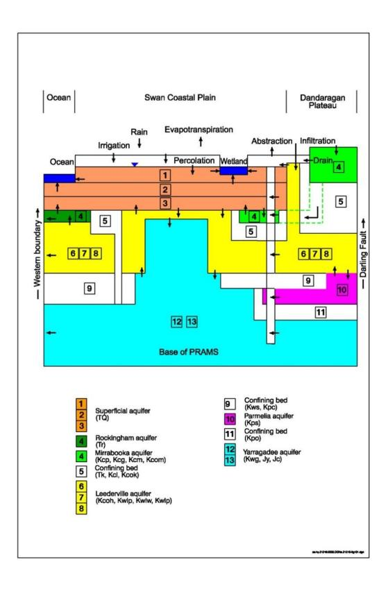
Figure 2: Conceptual Hydrogeological Model
