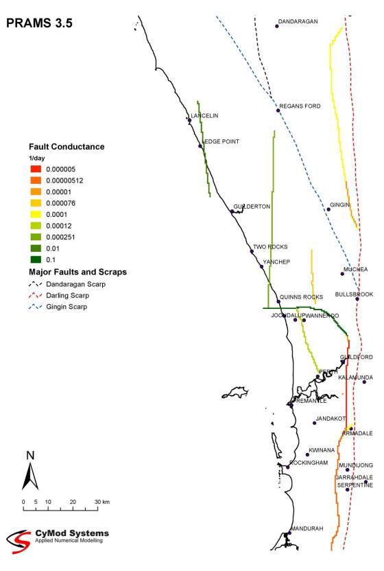
Figure 5: PRAMS 3.5A Faulting - Layers 6 through 8
