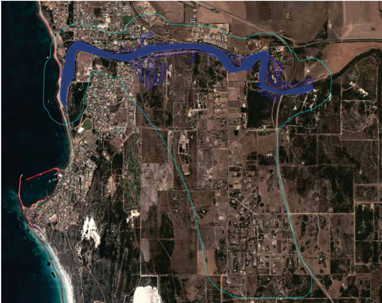
Figure 16 - 100 year floodplain (dark blue) and flood development control area (light blue). Source: Salim 1997.
