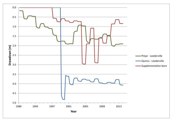
Figure 7-3 Transient simulation - potentiometric head drawdown, Layer 2 (Leederville aquifer) beneath Lake Nowergup.
