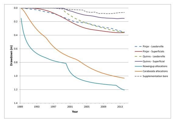
Figure 7-4 Transient simulation using zone of low hydraulic conductivity in Superficial aquifer west of Lake Nowergup - watertable drawdown, Layer 1 (Superficial aquifer) beneath Lake Nowergup.
