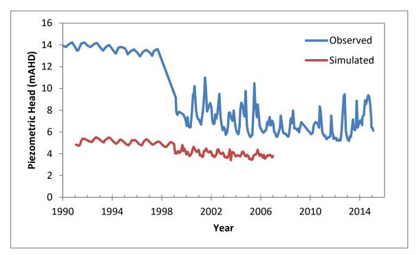
Figure 6-4 Observed and simulated head - Bore AM20A, Leederville Formation.
