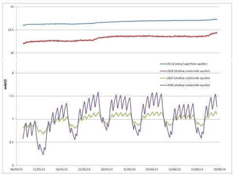
Figure 4-5 Data logger water levels for LN16, 18, 37 and 38 during May-June 2014.
