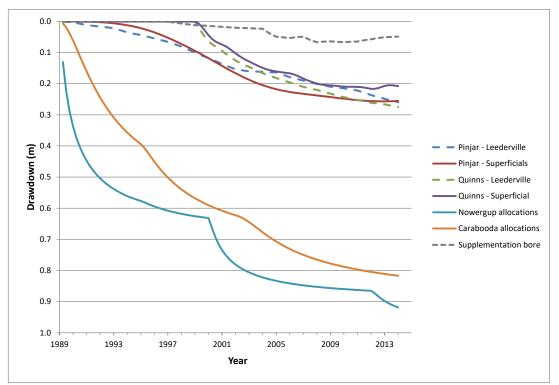
Figure 7-2 Transient simulation - watertable drawdown, Layer 1 (Superficial aquifer) beneath Lake Nowergup.
