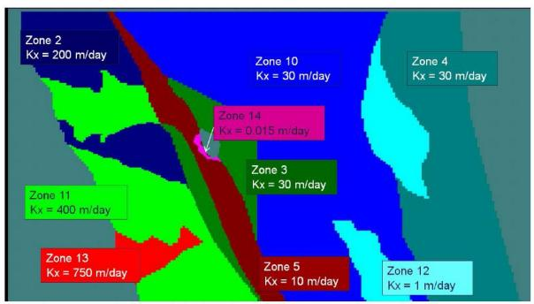
Note: In all zones Ky = Kx and Kz is one tenth of Kx (except for Zone 14 where Kx = 0.0015 and Kz = 0.015) Figure 6-2 Hydraulic conductivity distribution for the Superficial aquifer – Layers 1 to 5 (Figure 29 from SKM, 2009a).
