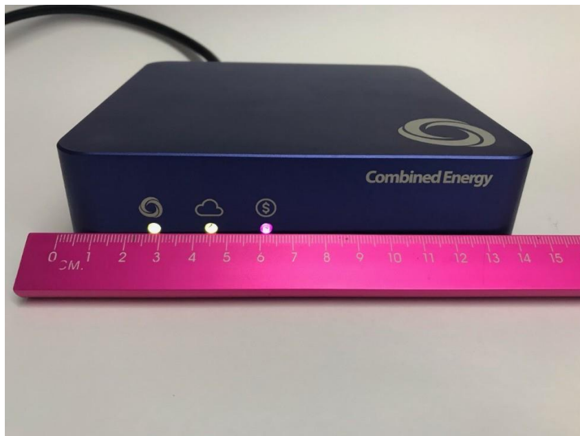
Figure 1 Self-install EMU edge gateway showing event programmable LEDs. Colour, activity (eg flashing) remotely programmable.
