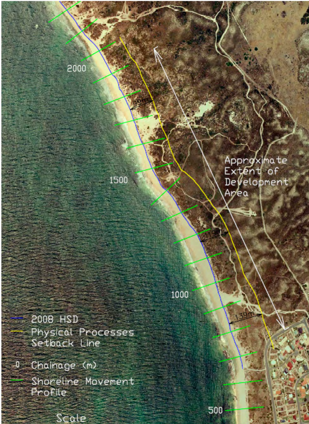
FIGURE 4.9 RECOMMENDED COASTAL SETBACK [SOURCE: MP ROGERS & ASSOCIATES]
