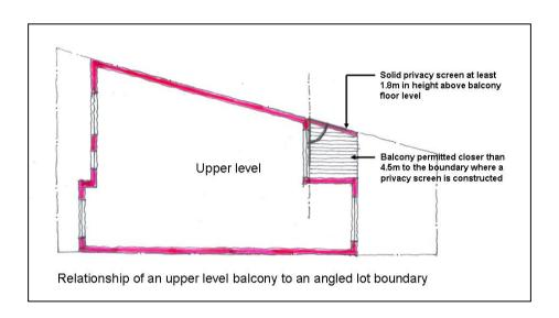
Where a balcony or deck at an upper level is located within 4.5m of a boundary with another lot, the balcony shall incorporate a permanent solid vertical screen to a height of 1.8m above the finished floor level on the side of the balcony facing the adjacent property.
