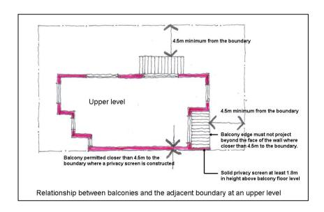
Balconies or decks at an upper level may be located within 4.5m of the boundary to an adjacent lot where the wall is equal to, or greater than, 75 degree to the boundary, provided that the balcony does not project beyond the face of the wall.
