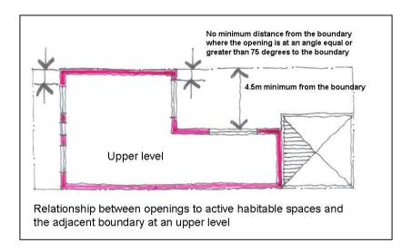
2 Major openings at all upper levels including the split levels may be located within 4.5 metres provided the sill level of the major opening is at least 1650mm above its finished floor level.
