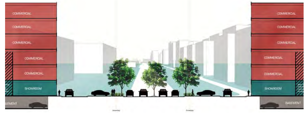
Figure 54. Boulevard Edge and Entry Streets (Note: This diagram does not specify building setbacks)
