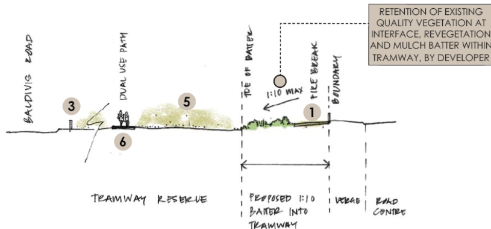
SECTION ABSTRACTED FROM Civil Group Dwg 7808-0-C510 Rev B, INDICATING BATTERING AND REVEGETATION
