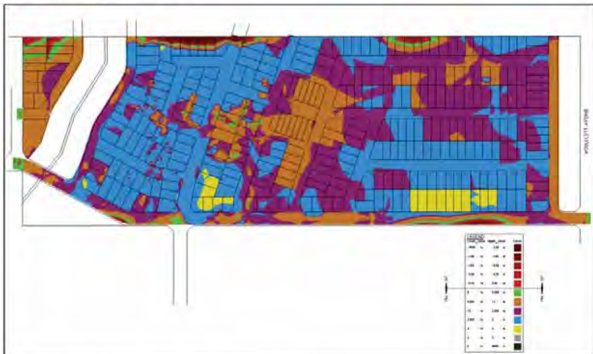
Figure 5: Site Bulk Earthworks and Cut/Fill area plans
