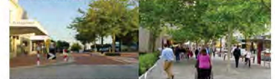
Change of carriage way pavement creates a pedestrian orientated environment, where car drivers naturally slow down; Angove Street, North Perth. An active street will naturally slow down car drivers, while an empty street gives no incentives to reduce speed
