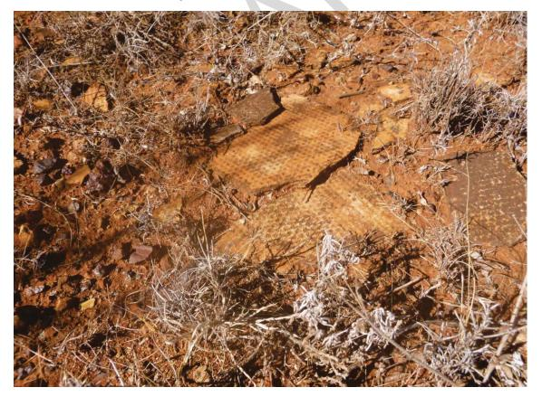
Plate 4. Widespread asbestos contamination on the surface soils of the site. Photograph is of sample location S1 in the north-west of the site.
