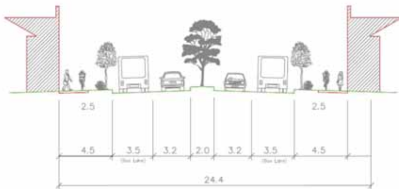
Figure 52: Wellington Road Proposed Cross-section (Walter Road West to Morley Drive)
