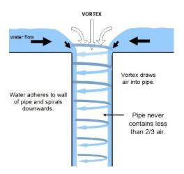
Figure 1 Conventional Gravity Fed down pipe.
