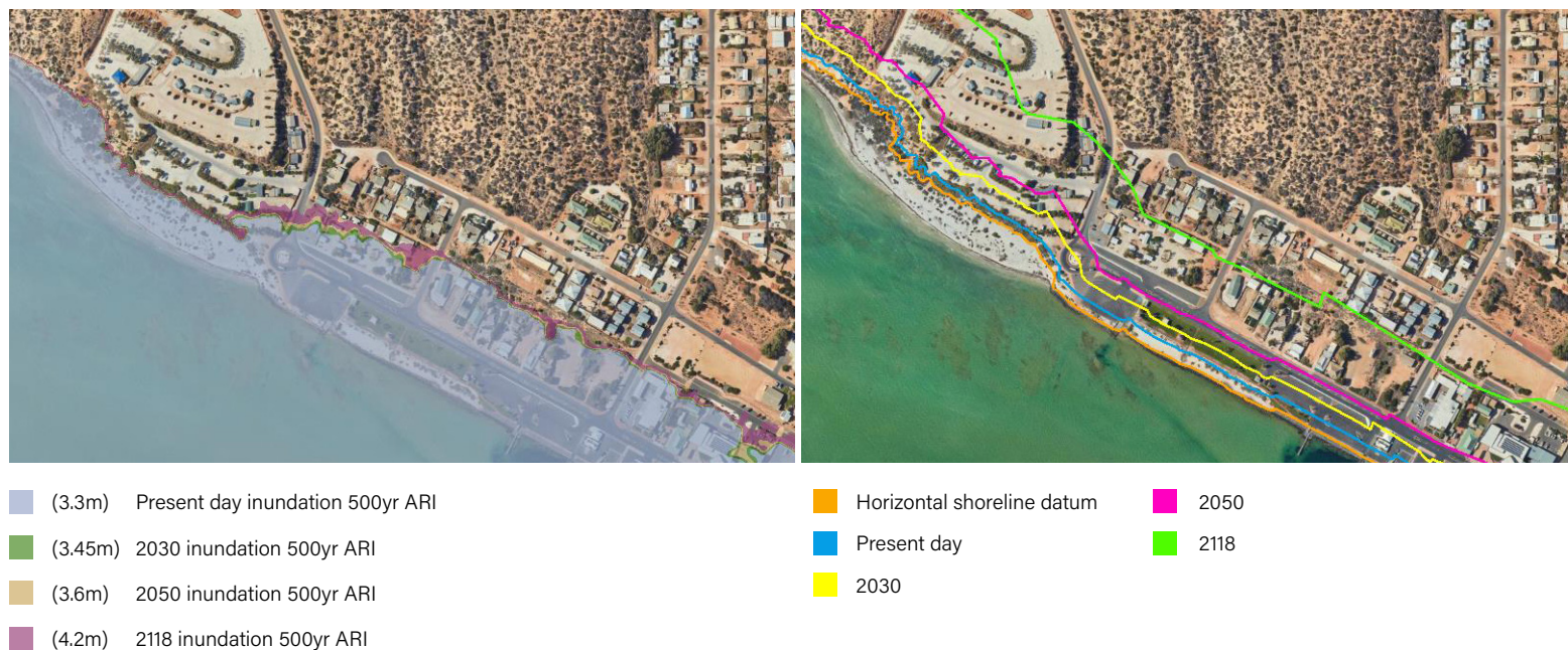
Figure 1: Example of coastal hazard mapping at Denham Townsite. Coastal inundation (left) and coastal erosion (right) modelled over a 100-year timeframe (2018 – 2118)
