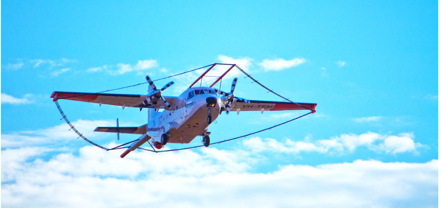
Image of airborne electromagnetic surveying
