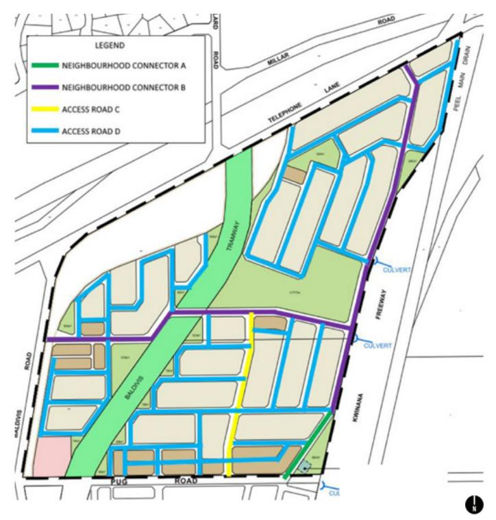
Figure 11 - Internal Road Hierarchy Source: Cardno
