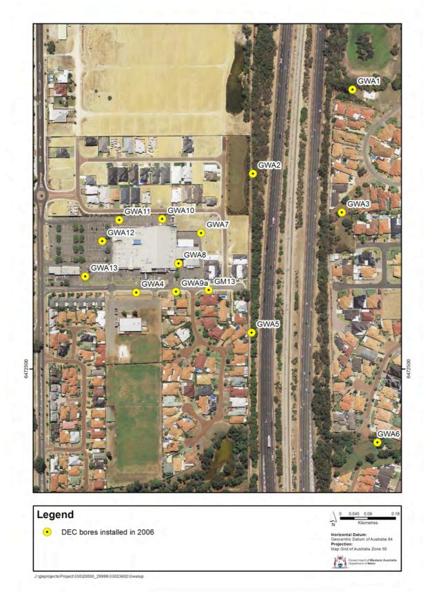
Figure 17 Location of groundwater bores installed by DEC in 2006
