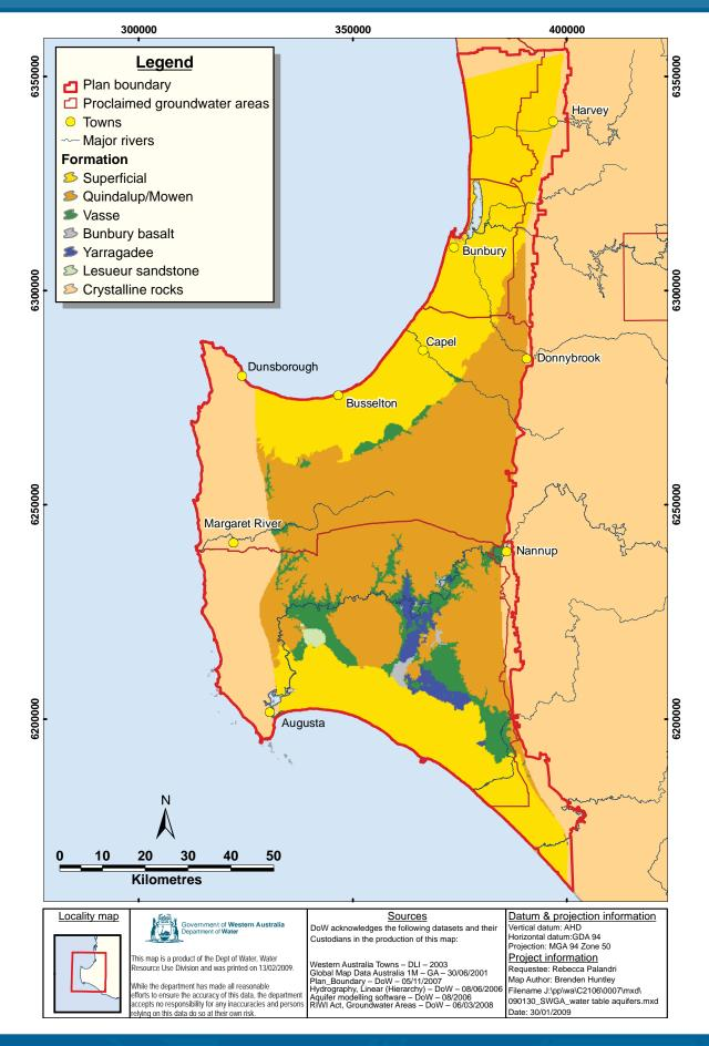
Figure 3 Surface hydrogeology of the plan area
