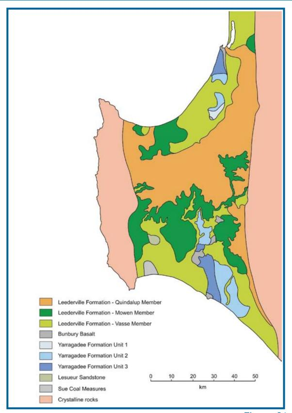
Figure A1 Geological diagram showing distribution of Leederville Formation and older formations
