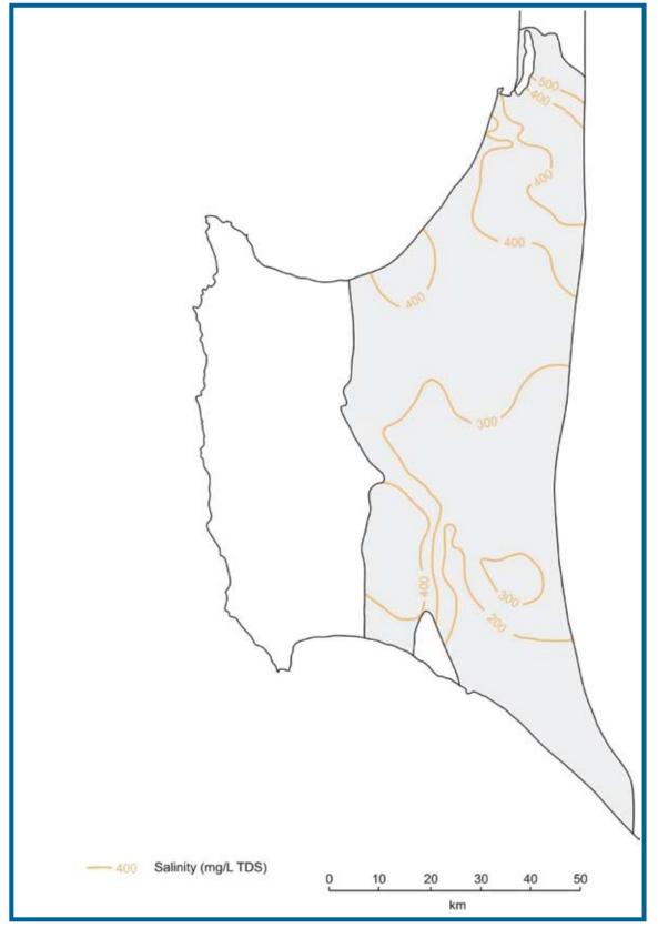
**Figure A3** Diagram of groundwater salinity in the Yarragadee Aquifer
