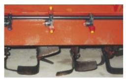
Use of rotary hoes is poor management practice because fast rotation speed pulverises the topsoil and the broad blades smear and seal the subsoil.
