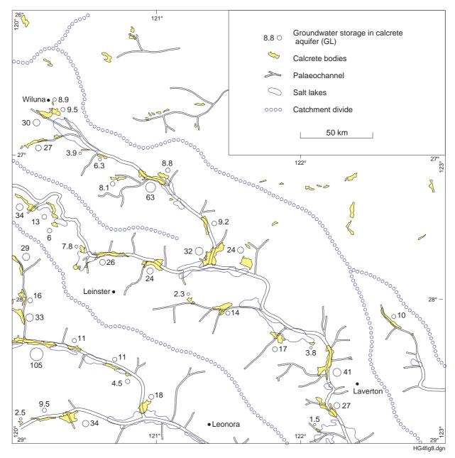
Figure 8. Groundwater storage in calcrete
