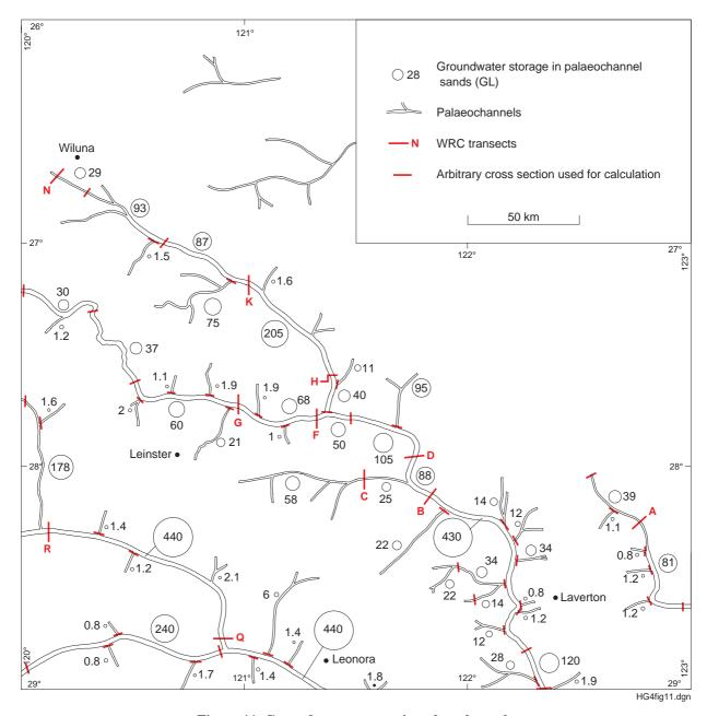
Figure 11. Groundwater storage in palaeochannels
