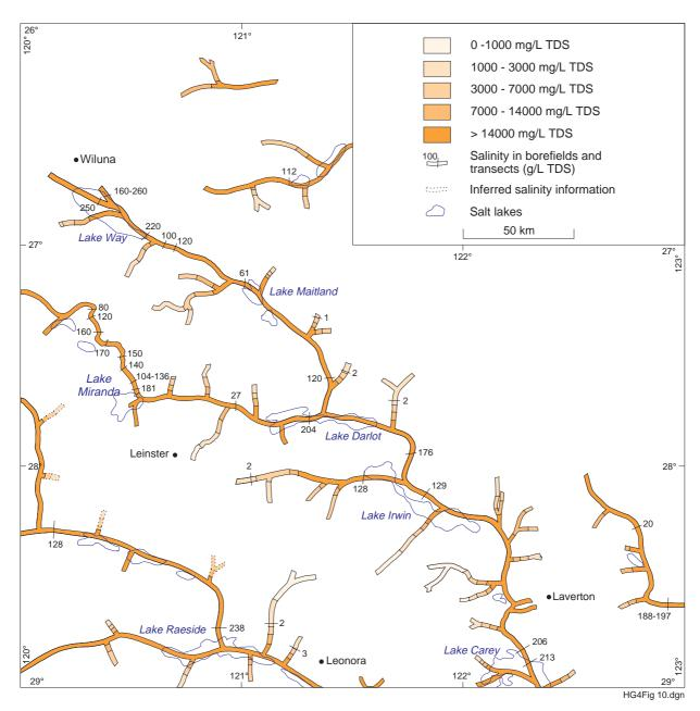
Figure 10. Groundwater salinity - palaeochannels
