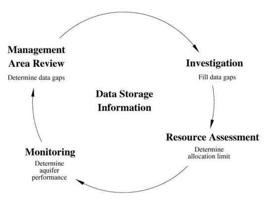
Figure 3. The groundwater resource assessment process
