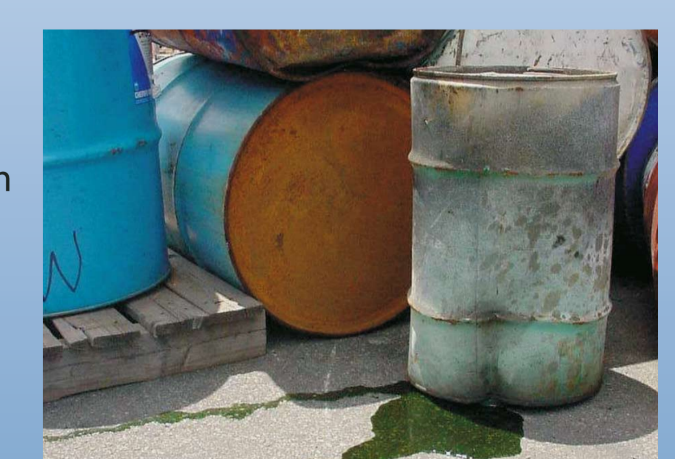
Leaking chemicals due to poor storage (courtesy of Department of Environment).
