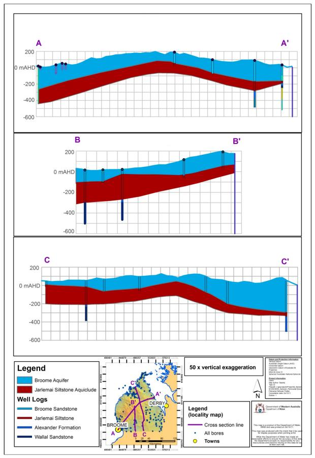
Figure 9 Schematic hydrogeological sections
