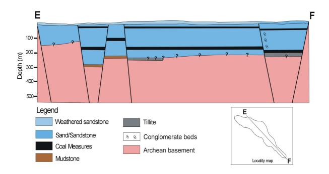
Figure 4. Geological cross-section of Wilga Basin East
