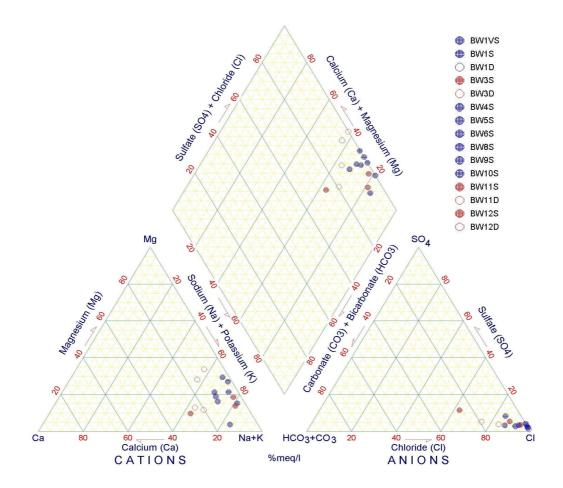
Figure 9. Trilinear diagram of major ion chemistry
