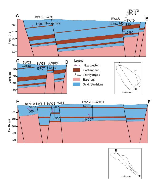
Figure 5. Hydrogeological cross-sections of Wilga Basin West and East
