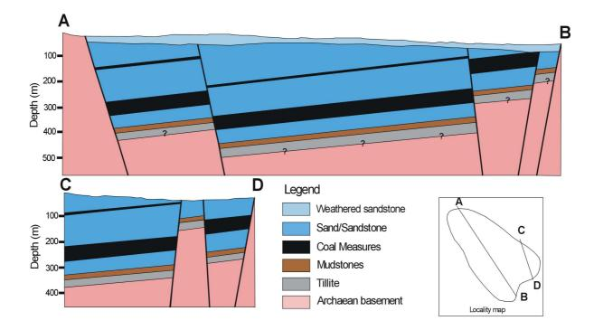
Figure 3. Geological cross-section of Wilga Basin West
