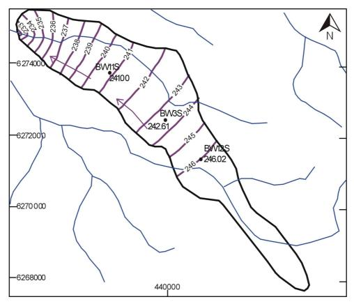
Figure 7. Watertable contours for Wilga Basin East (m AHD)
