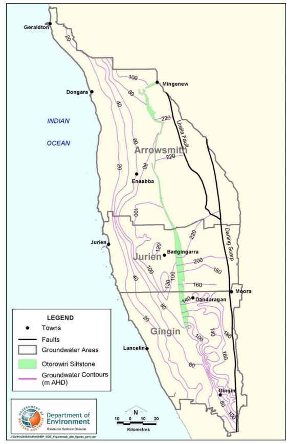
Figure 6: Watertable configuration in the Northern Perth Basin
