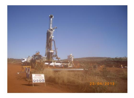
Figure B3 Pump testing of a bore drilled in the new Homestead Bore field, photograph by J. Kaub
