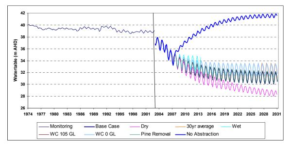
Figure 70 Observed and predicted hydrographs for eight modelling scenarios at monitoring bore WM28
